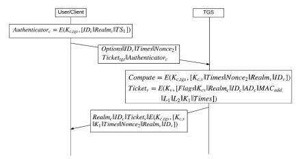
Figure 4. The Client/Server Authentication Exchange Phase
